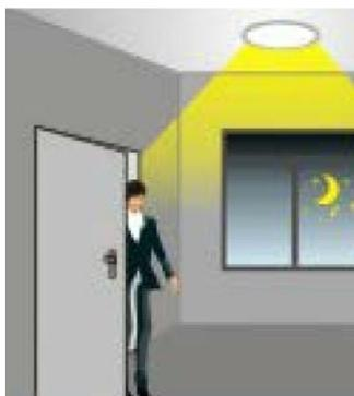
With sufficient ambient light, the sensor switches on the lamp when motion is detected.
