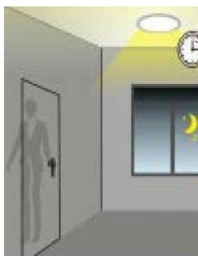
After hold time the lamp gradually dims down if no motion is detected.
