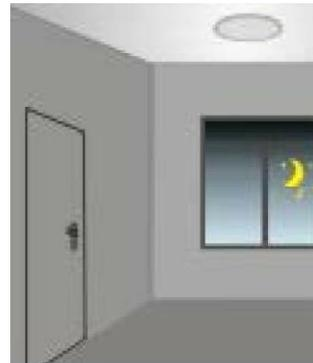
After standby period the sensor switches off the lamp if no motion is detected in its detection zone.
