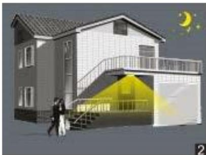
With sufficient ambient light, the sensor switches on the lamp when motion is detected.
